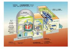
Fig. 7. Bird's-eye view of MSR-FUJI.
